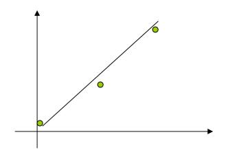
Select a curve that best fit the data. One choice is find the curve so that the sum of the square of the error is minimized.
