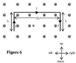
Q15. A segment of wire carries a current of 25 A. It is bent into the shape shown in Figure 4. The wire is placed in a uniform magnetic field of 40 mT and directed out of the page. Find the magnitude of the magnetic force on this segment of wire. Ans:5.0 N
