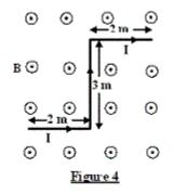
Q16. Two infinite wires are parallel to the y-axis. One carries current i1 = 12 A in the +y-axis at x=0; the other carries i2 at x = 8.0 cm. For what magnitude and direction of i2 will the resultant magnetic field be zero at x = 6.0 cm?Ans:4.0 A in the +y-axis.
