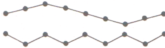
Transverse waves in a one-dimensional lattice.
