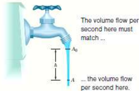
Figure 14-18 As water falls from a tap, its speed increases. Because the volume flow rate must be the same at all horizontal cross sections of the stream, the stream must “neck down” (narrow).
