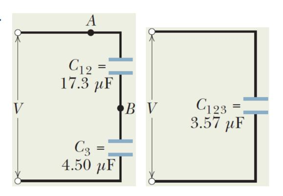
(b) The potential difference applied to the input terminals in the figure is  $V=12.5\,\mathrm{V}$ . What is the charge on  $C_1$ ?
