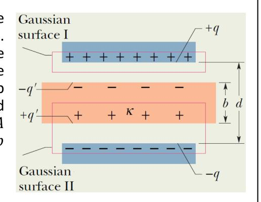
(a) What is the capacitance  $C_0$  before the dielectric slab is inserted?
