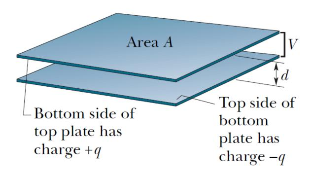
When a capacitor is *charged*, its plates have charges of equal magnitudes but opposite signs: +q and -q. However, we refer to the *charge of a capacitor* as being q, the absolute value of these charges on the plates.
