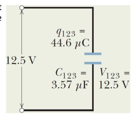
The charge on capacitors  $C_{12}$  and  $C_3$  is the same as that on capacitor  $C_{123}$ :
