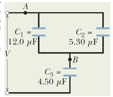
Now capacitors  $C_{12}$  and  $C_3$  are in series. Their equivalent capacitance  $C_{123}$  is
