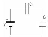
**Q17.:** Figure (7) shows three capacitors connected to a battery of voltage V = 6 Volts. The charges on the capacitors are known to be  $Q_1 = 24 \mu C$  for  $C_1$  and  $Q_2 = 96 \mu C$  for  $C_2$ . What are the values of the capacitances  $C_1$  and  $C_2$ ? (Ans: C1=8  $\mu$ F, C2= 16  $\mu$ F)
