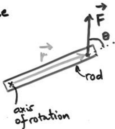
The force  $\vec{F}$  will make the rod rotate.
