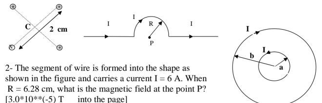
3- The figure shows two concentric circular loops of radii a and b and both carry a current I. Find the resultant magnetic field at the center of the two loops if a = 10 cm, b = 20 cm and I = 20 A. [63 micro-T, out of the page]
