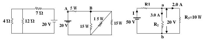
7- What is the power dissipated in the 4.0-Ohm resistor in the figure. [9.0 W]
