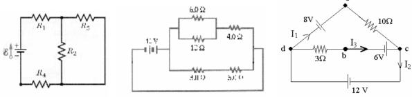
2- The current in the 5.0-ohm resistor in the circuit shown in the figure is: [5.0 A]
