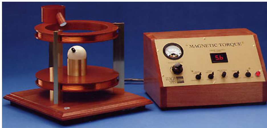
Figure 3: The M\tau instrument used to simulate the Larmor frequency.
