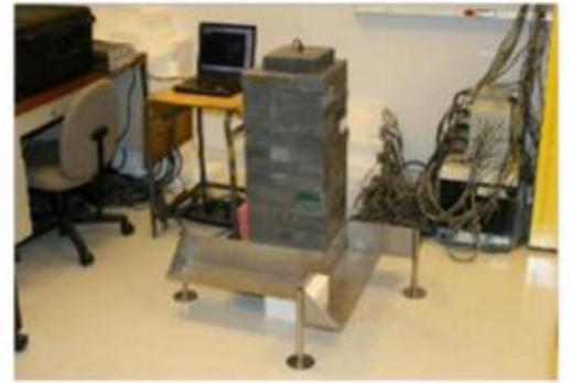
Figure 3. Background and self-activity gamma-ray spectra are acquired at UNLV using this "UNLV Lead Shielding Pyramid."
