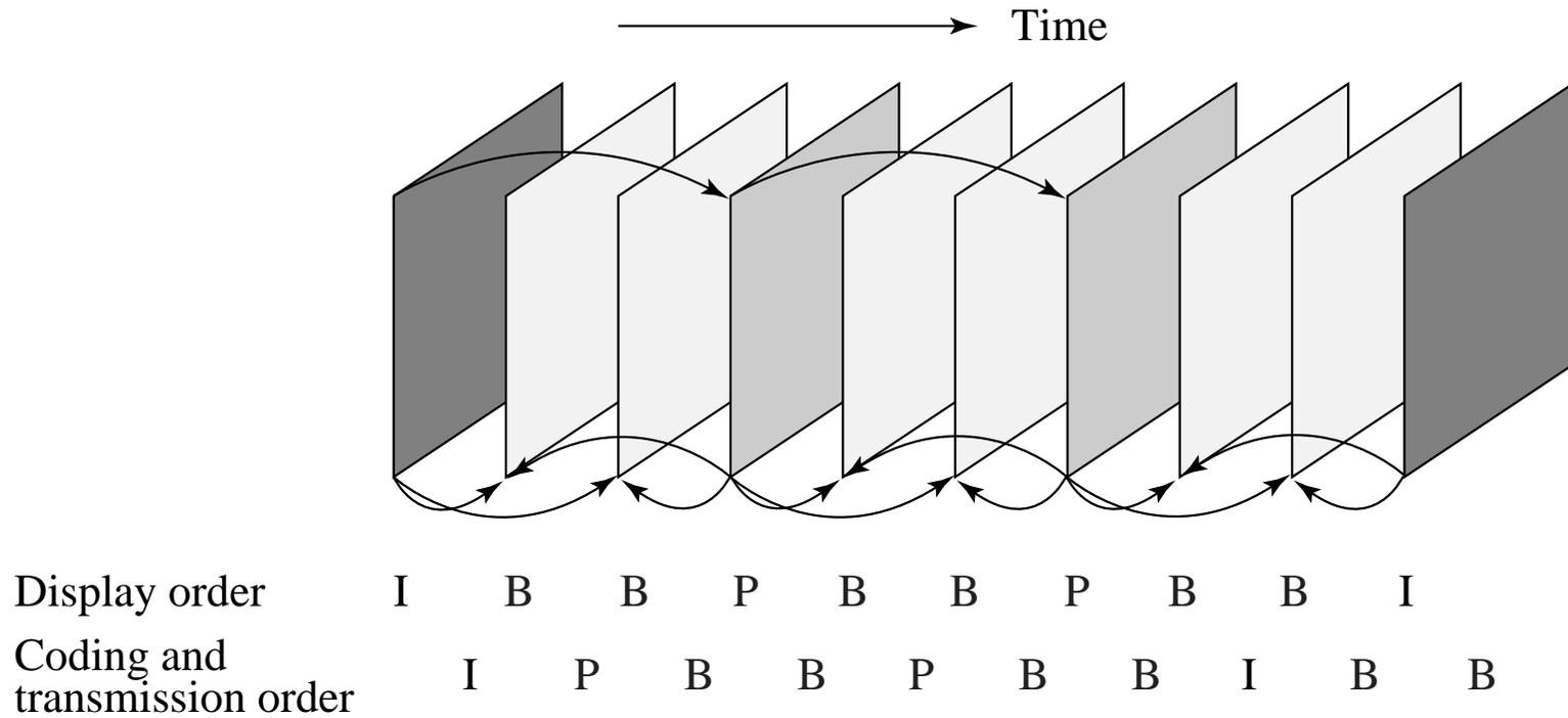
Fig 11.3: MPEG Frame Sequence.
