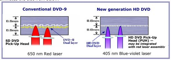
Although the data density is much greater in HD DVD discs, the structure is very similar to existing DVDs. Discs may be single or double-sided, giving a total storage potential of 60GB on a single disc.
