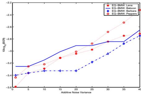
Figure 6: Logarithmic BERs of BCH (15, 7) code in the presence of AWGN noise using watermark length of 256 bits.
