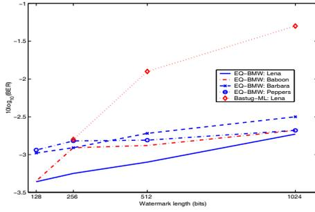
Figure 5: Logarithmic BERs of repetition-coding using BMW method and block DCT for various watermark lengths ( $M = 128, 256, 512,$  and  $1024$ ).
