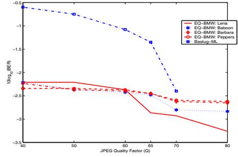
Figure 7: Logarithmic BERs of BCH (15, 7) code in the presence of JPEG compression using watermark length of 256 bits.
