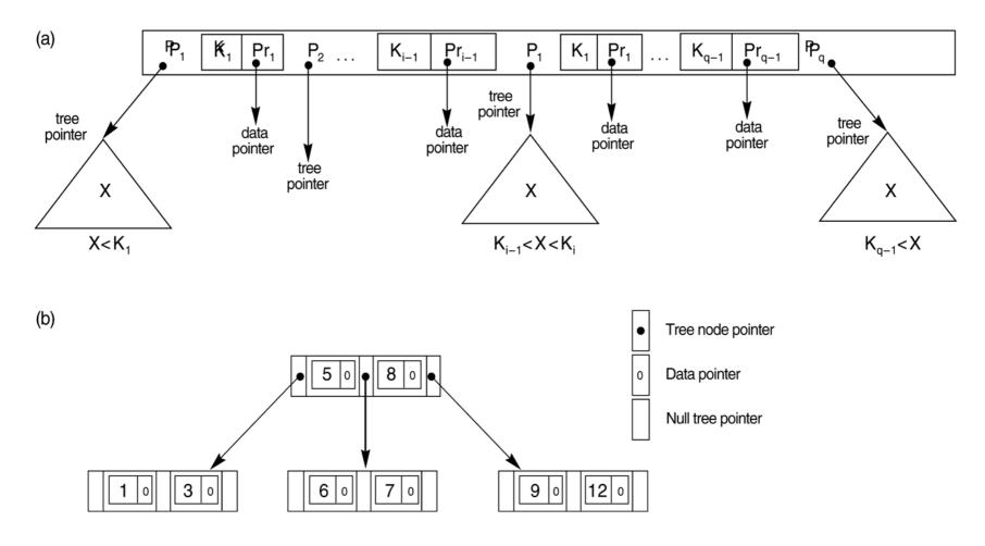
The nodes of a B+-tree. (a) Internal node of a B+-tree with q -1 search values. (b) Leaf node of a B+-tree with q - 1 search values and q - 1 data pointers.
