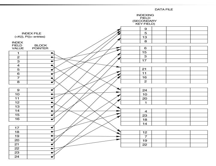
A secondary index (with recored pointers) on a nonkey field implemented using one level of indirection so that index entries are of fixed length and have unique field values.
