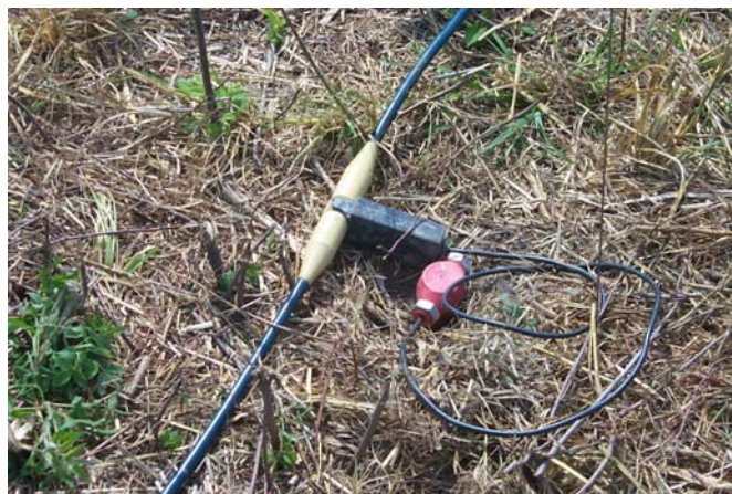
4.5 Hz geophone with spikes connected to 4 ft takeout, 60-pair seismic cables.
