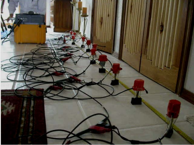
Small scale ReMi geophone array setup to evaluate fill conditions under concrete slab. Binder clips were set on spikes and then taped to the geophone bodies for mounting on the floor (Picture from the paper of Michael Rucker).
