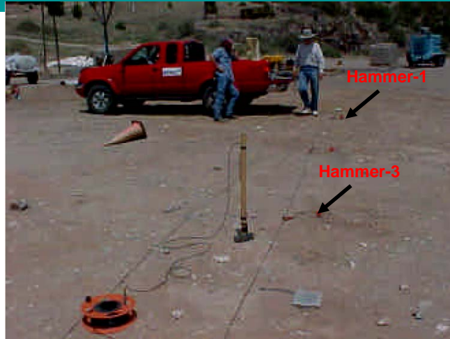
Combined ReMi and seismic refraction setup in Sandia Mountains, NM. Equipment is set up on the back of the truck. Geophone spacing is 10 feet and the array length is 120 feet. The author is beginning to jog to generate surface waves for a ReMi data set; the sledge hammer seismic refraction energy source is in the foreground. (Figure 1, Michael Rucker's paper).
