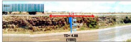
Figure 2. Example ITM interpretation with apparent depth of investigation from optimization interpretation. Upper photo shows exposed limestone at the proposed excavation cut. The center plot shows the ITM and depth of investigation interpretation. The lower plot shows the time-distance plots for the seismic first arrival data. Project units are metric, and seismic wave velocities are in meters per second (m/s).
