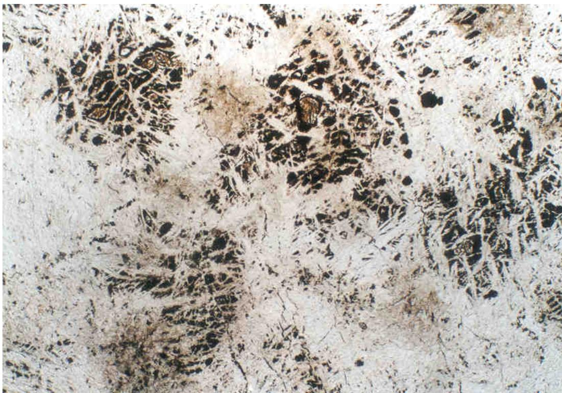
Figure 4. Thin section photograph for the serpentinite showing the mesh textures (X10).
