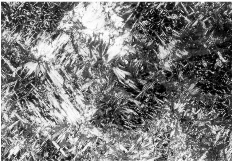
Figure 3. Thin section photograph showing the relict textures of the altered pyroxene within the serpentinite (X10)
