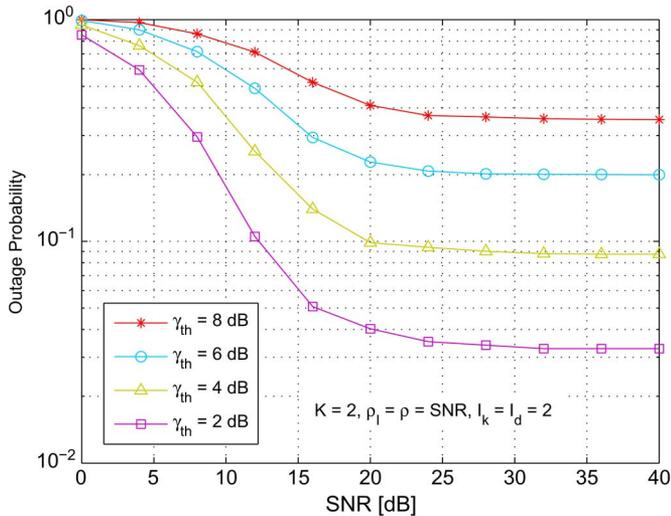
Fig. 7. Outage probability versus average SNR of the opportunistic DF relaying system with two relays for different values of outage threshold. We have set  $m_{s,d} = 1$ ,  $\sigma_{s,d}^2 = 1$ ,  $m_{s,k} = m_{k,d} = k$  for  $k = 1, 2$ ,  $\sigma_{s,1}^2 = \sigma_{s,2}^2 = 0.2$ ,  $\sigma_{1,d}^2 = 0.4$ ,  $\sigma_{2,d}^2 = 0.6$ ,  $m_1^I = m_2^I = 2$ ,  $(\sigma_k^I)^2 = (\sigma_d^I)^2 = 0.1$ , and  $m_d^I = 1$ .
