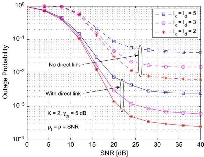
Fig. 3. Outage probability versus average SNR of the opportunistic DF relaying system with two relays for different number of interferers at the relays and the destination. We have set  $m_{s,d} = 1$ ,  $\sigma_{s,d}^2 = 1$ ,  $m_{s,k}$  and  $m_{k,d} = k$  for  $k = 1, 2$ ,  $\sigma_{s,1}^2 = \sigma_{s,2}^2 = 0.2$ ,  $\sigma_{1,d}^2 = 0.4$ ,  $\sigma_{2,d}^2 = 0.6$ ,  $m_1^I = m_2^I = 1$ ,  $(\sigma_k^I)^2 = (\sigma_d^I)^2 = 0.01$ , and  $m_d^I = 1$ .
