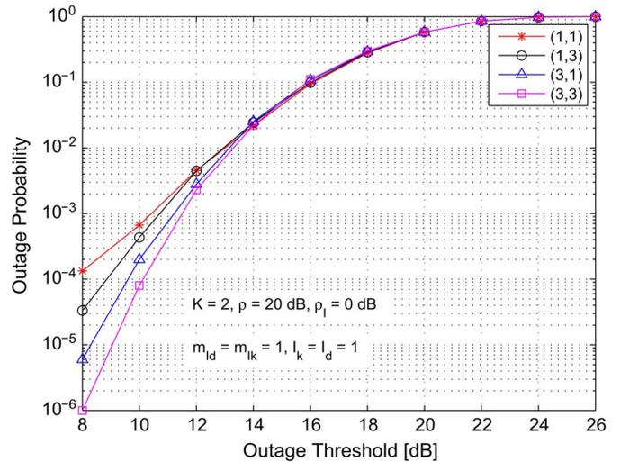
Fig. 5. Outage probability versus outage threshold of the opportunistic DF relaying system with two relays for different values of fading parameters  $(m_{s,k}, m_{k,d})$ . We have set  $m_{s,d} = 3$ ,  $\sigma_{s,d}^2 = 1$ ,  $\sigma_{s,1}^2 = 0.2$ ,  $\sigma_{1,d}^2 = 0.4$ ,  $\sigma_{s,2}^2 = 0.2$ ,  $\sigma_{2,d}^2 = 0.6$ , and  $(\sigma_k^I)^2 = (\sigma_d^I)^2 = 0.01$ .
