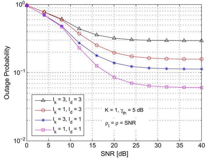
Fig. 4. Outage probability versus average SNR of the opportunistic DF relaying system with one relay for different number of interferers at the relay and the destination. We have set  $m_{s,d} = 1$ ,  $\sigma_{s,d}^2 = 1$ ,  $m_{s,1} = 1$ ,  $m_{1,d} = 2$ ,  $\sigma_{s,1}^2 = 0.2$ ,  $\sigma_{1,d}^2 = 0.4$ ,  $m_1^I = 1$ ,  $(\sigma_1^I)^2 = (\sigma_d^I)^2 = 0.05$ , and  $m_d^I = 1$ .
