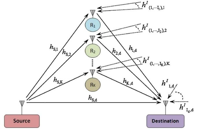
Fig. 1. Dual-hop opportunistic DF relaying system with CCI at both the relay and the destination.
