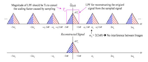
If the signal was sampled at a sampling rate lower that 2 times the bandwidth of the signal (called the **NYQUIST SAMPLING RATE**), the different spectral components of the sampled signal (called IMAGES) will interfere with each other and reconstructing the original signal will be impossible. This is illustrated in the following figure. The dark parts in the figure represent parts of the sampled signal and reconstructed signal that have been damaged.
