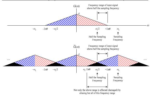
So, it is clear that not only the range of the input signal  $[\omega/2, 2\pi B]$  gets affected by aliasing, but all the range from  $[\omega/2\pi B]$  is affected by aliasing.
