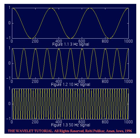
So how do we measure frequency, or how do we find the frequency content of a signal? The answer is **FOURIER TRANSFORM (FT)**. If the FT of a signal in time domain is taken, the frequency-amplitude representation of that signal is obtained. In other words, we now have a plot with one axis being the frequency and the other being the amplitude. This plot tells us how much of each frequency exists in our signal.
