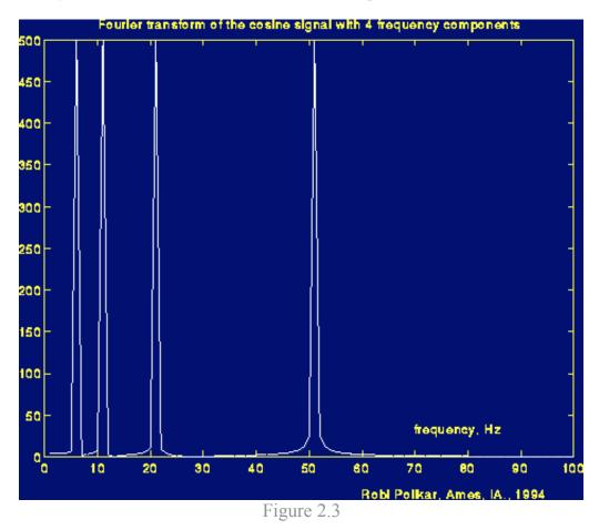
Note the four peaks in the above figure, which correspond to four different frequencies.
