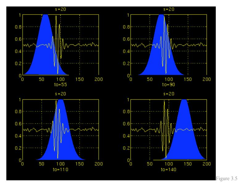
Figures 3.4 and 3.5 illustrate the same process for the scales s=5 and s=20, respectively. Note how the window width changes with increasing scale (decreasing frequency). As the window width increases, the transform starts picking up the lower frequency components.
