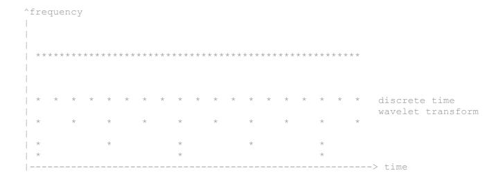
In discrete time case, the time resolution of the signal works the same as above, but now, the frequency information has different resolutions at every stage too. Note that, lower frequencies are better resolved in frequency, where as higher frequencies are not. Note how the spacing between subsequent frequency components increase as frequency increases.
