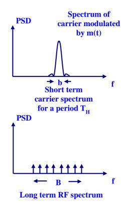
The various network carriers follow different trajectories on the grid. Only the carrier whose trajectory coincides with that regenerated by the local synthesizer will be demodulated.
