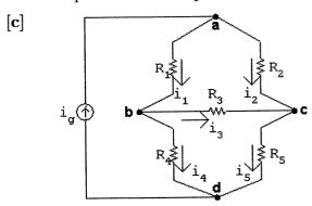
Sum the currents at any three of the four essential nodes a, b, c, and d. Using nodes a, b, and c we get
