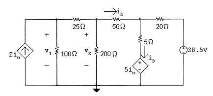
$$i_o = \frac{v_2 - v_3}{50}$$
