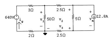
$$\frac{v_1}{50} + \frac{v_1 - 640}{5} + \frac{v_1 - v_2}{2.5} = 0 \qquad \text{so} \qquad 31v_1 - 20v_2 + 0v_3 = 6400$$
