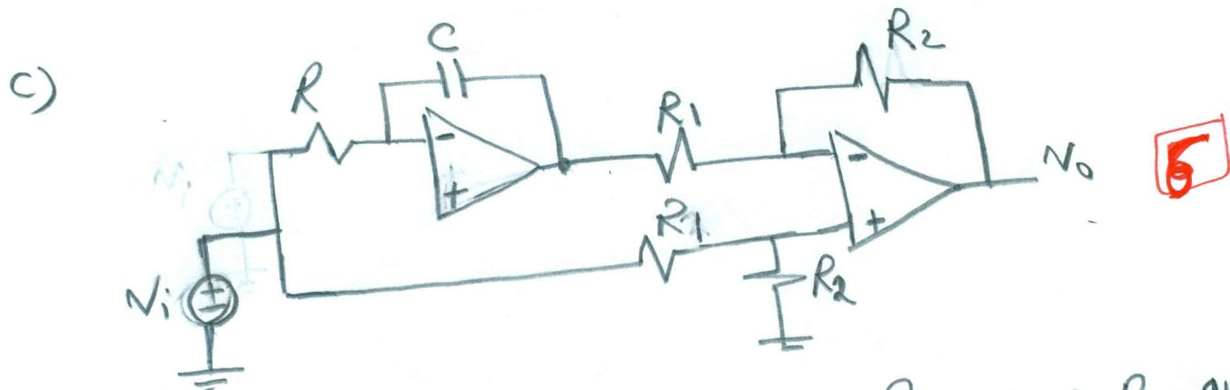
$$v_o = \frac{1}{RC} \left( \frac{R_2}{R_1} \right) \int v_i dt + \frac{R_2}{R_1} v_i \Rightarrow \frac{R_2}{R_1} = 2 \Rightarrow R_2 = 2k \quad R_1 = 1k$$
