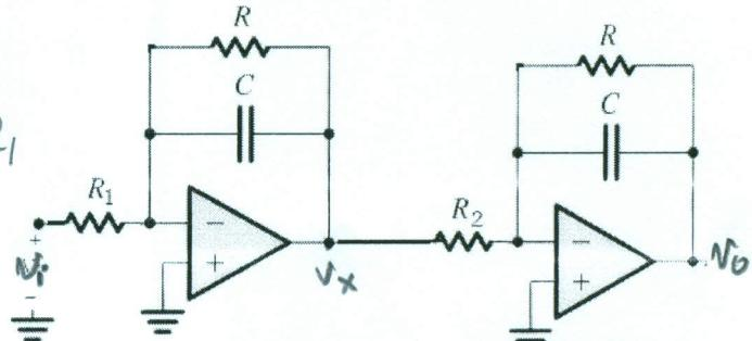
$$= \frac{R^2}{s^2 C^2 R^2 R_1 R_2 + 2sCR_1 R_2 + R_1 R_2} = \frac{\frac{1}{C^2 R_1 R_2}}{s^2 + 2s\frac{1}{CR} + \frac{1}{C^2 R^2}}$$
