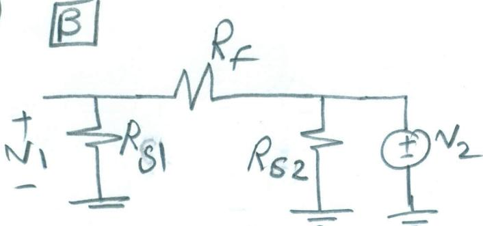
$$\beta = \frac{N_1}{N_2} = \frac{R_{S1}}{R_{S1} + R_F} \quad \boxed{6}$$
