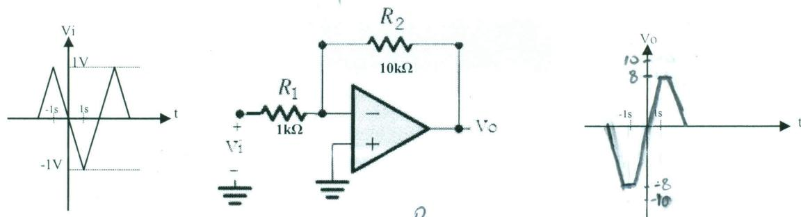
$$\text{Gain} = -\frac{R_2}{R_1} = -10$$
