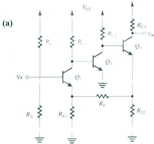
$$\beta = \frac{N_1}{Z_2} = \frac{R_{E2} R_{E1}}{R_{E2} + R_F + R_{E1}} \quad \boxed{6}$$
