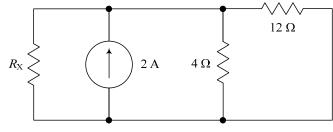
(11) Find  $R_{\rm L}$  that will absorb the maximum power from the circuit (DO NOT find the maximum power).
