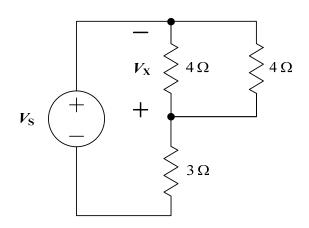
(2) Using current division in the circuit below, we find that  $I_X$  is equal to:
