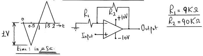
The amplifier has an offset voltage = 2 mV, biasing currents = 1 uA and 1.5 uA and slew-rate = 1.0 V/1.0 usec.
