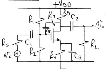
C1=C2=10MF, Rs=100S, R=R2=10MS, Rs=5K, Ry=1K, C3=100MF, R3=100KS, C5=20MF, RL=10K.
