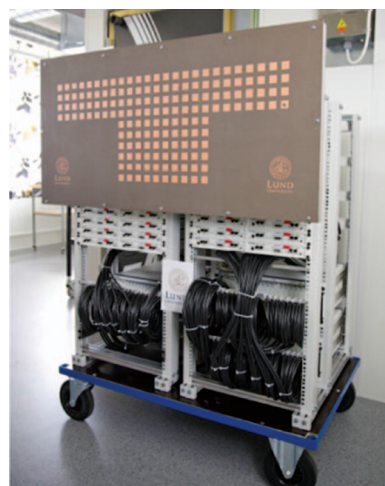
FIGURE 8. A 100-element massive-MIMO antenna system and test bed [30].
