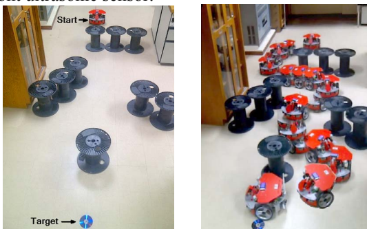
Figure-10: Environment along with the path generated to the target using only the front ultrasonic sensor.
