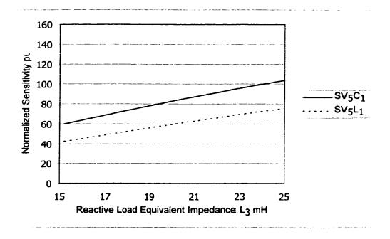
Figure 5.9: Parametric Sensitivities versus Reactive Load Equivalent
