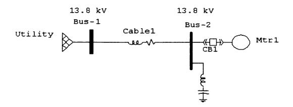
Figure 5.10: Single Line Diagram for Case Study 2 (De-tuned Capacitor)
