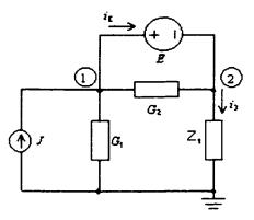
Figure 3.4 Introduction of  $i_E$  and  $i_3$  as new variables
