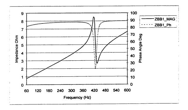
Figure 5.20 Impedance Frequency Scan For Bus # bb1
