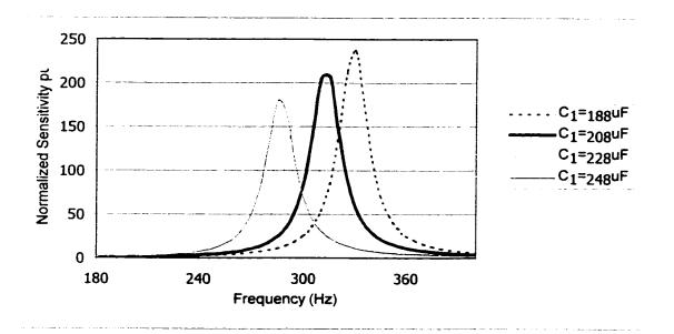
Figure 5.6: Parametric Sensitivities versus Frequency as the PFC Capacitance (C1)
