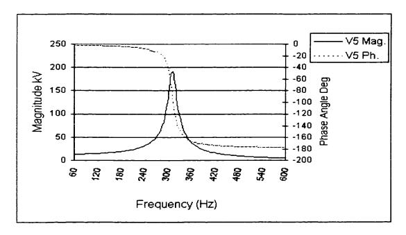
(Case 1: Radial System With a Plain PFC Capacitor)
