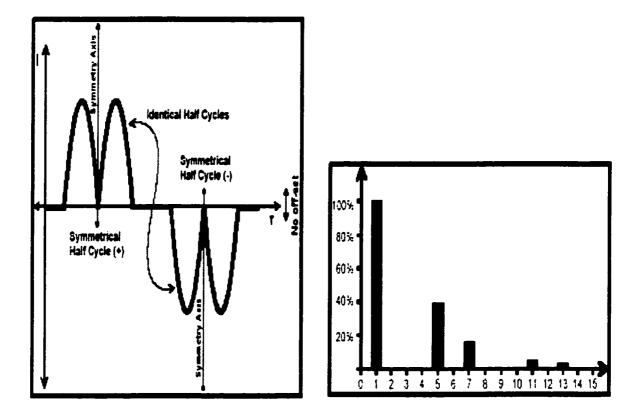
Figure 1.3: Line Current Three-Phase Converter and its Harmonic Spectrum.
