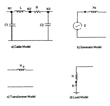
Figure 5.19: Typical Equivalent Power System Elements Models for MNFSA
