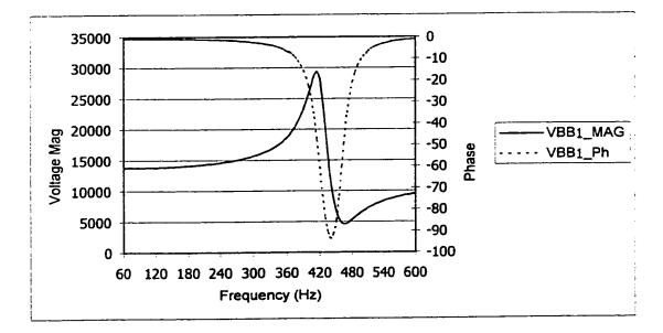
Figure 5.21 Voltage Frequency Response at Bus # bb1
