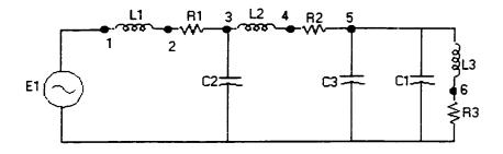
Figure 5.2 : Circuit Diagram for Case Study 1 (Plain PFC)
