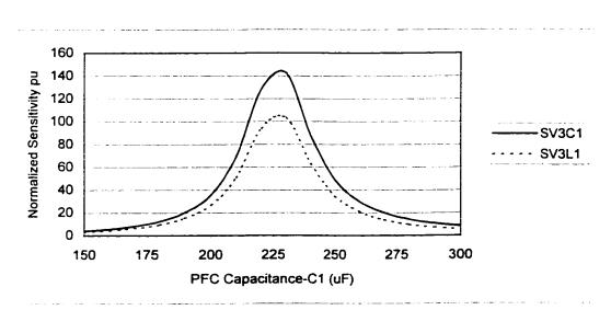
Figure 5.8: Parametric Sensitivities versus PFC Capacitance
