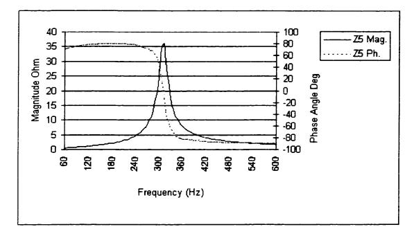
Figure 5.3: Impedance Frequency Scan at Node 5
