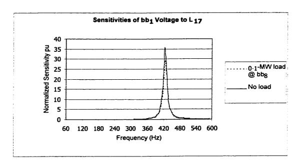
Figure 5.26 Sensitivity of Bus#bb1 Voltage to Parameter  $L_{17}$  With and Without
