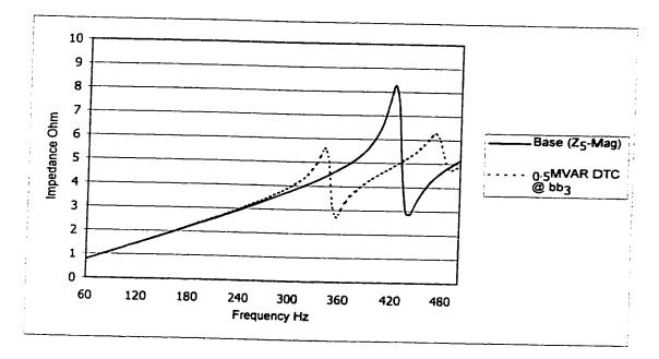
Figure 5.35 Frequency Scan at Bus # bb 1
