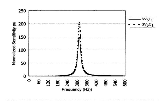
Figure 5.5: Parametric Sensitivities of Node 5 Voltage versus Frequency (Case 1: Radial System With a Plain PFC Capacitor)
