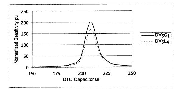
Fig 5.16: Parametric Sensitivities versus DTC Capacitance at 130 HZ L<sub>4</sub> is Fixed (Node 5 For Case 2)
