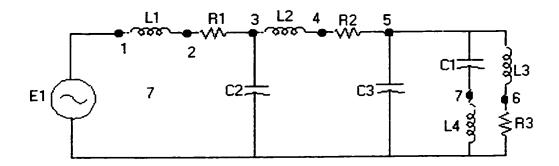
Figure 5.11: Circuit Diagram For Case Study 2 (De-Tuned Capacitor)
