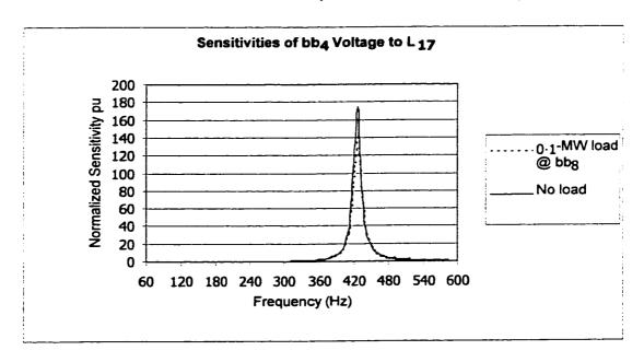
the 0.1 MW Load at Bus#bb8 (Case 4: 14 Bus Industrial System)
