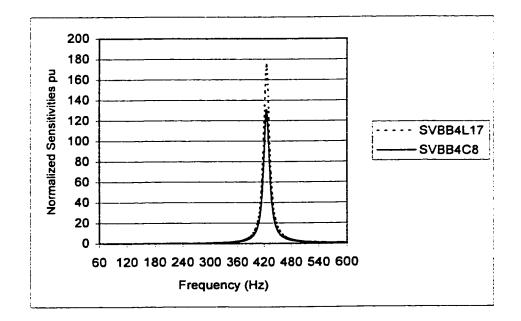
Figure 5.23 Parametric Sensitivities Versus Frequency For # bb4
