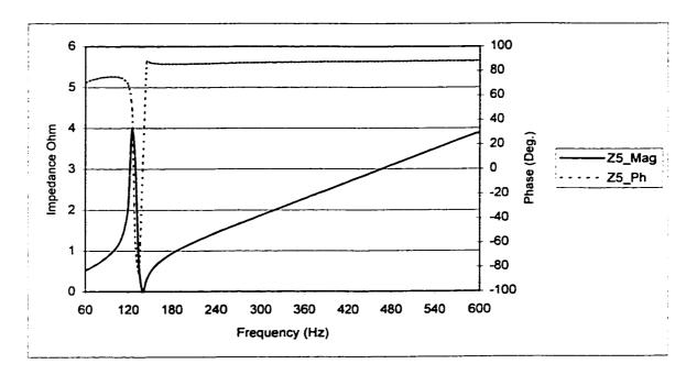
Figure 5.12 Impedance Frequency Scan For Node 5
