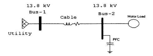
Figure 5.1 : Single Line Diagram for Case Study 1 (Plain PFC)
