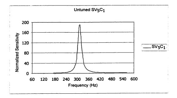
Figure 5.14: Parametric Sensitivities versus Frequency Un-Tuned System (Node 5 Voltage For Case 2)
