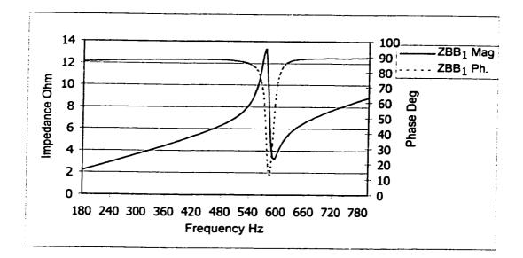
Figure 5.31 Impedance Frequency Scan For Bus # bb1
