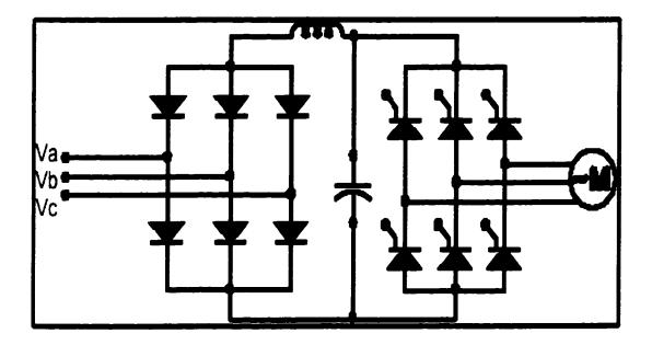
Figure 1.2 A: Three-Phase Power Converter
