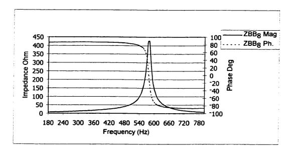
Figure 5.33 Impedance Frequency Scan For Bus # bb8
