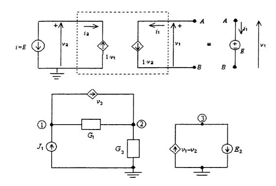
Figure 3.3 (a) Use of gyrator for ideal voltage source simulation, (b) Implementation of the gyrator.
