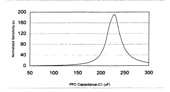
Figure 5.7: Parametric Sensitivities versus PFC Capacitance While the Frequency is Fixed at 300 Hz (Node 5 For Case 1)
