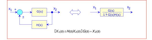
The utility of the block diagram transformation will be illustrated by an example using block diagram reduction.
