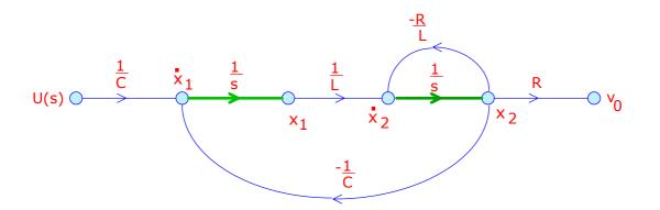
Using Mason's signal-flow gain formula, we may obtain the transfer function
