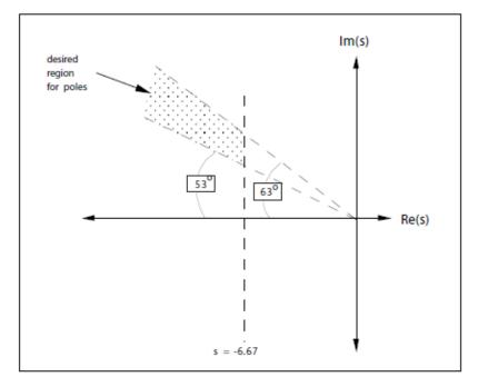
FIGURE P5.2 Desired region for pole placement.
