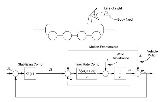
A communication antenna is mounted on a moving vehicle. It is required to precisely regulate the antenna line of sight event though the vehicle is subjected to significant pitching motion and the antenna is subjected to wind loads.
