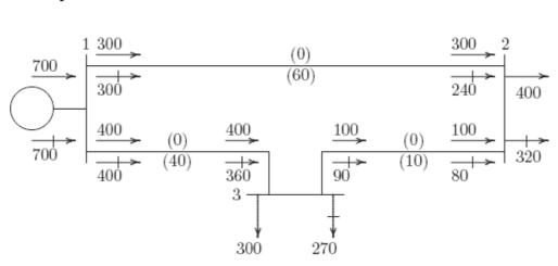
FIGURE 53 Power flow diagram of Problem 6.7 (powers in MW and Mvar).
