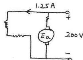
(c)  $E_a = V_t + I_a R_a = 200 + 100 \times 0.1 = 210 \text{ V}$
