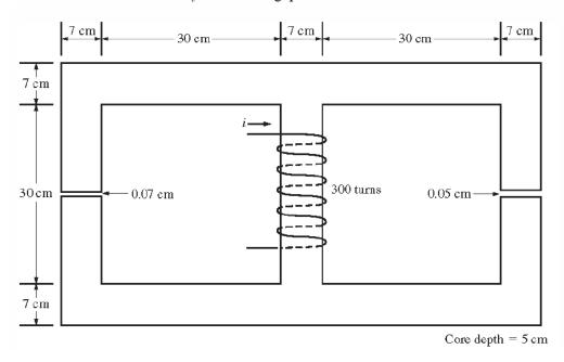
SOLUTION This core can be divided up into five regions. Let  $\mathcal{R}_1$  be the reluctance of the left-hand portion of the core,  $\mathcal{R}_2$  be the reluctance of the left-hand air gap,  $\mathcal{R}_3$  be the reluctance of the right-hand portion of the core,  $\mathcal{R}_4$  be the reluctance of the right-hand air gap, and  $\mathcal{R}_5$  be the reluctance of the center leg of the core. Then the total reluctance of the core is
