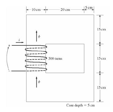
Solution There are three regions in this core. The top and bottom form one region, the left side forms a second region, and the right side forms a third region. If we assume that the mean path length of the flux is in the center of each leg of the core, and if we ignore spreading at the corners of the core, then the path lengths are  $l_1 = 2(27.5 \text{ cm}) = 55 \text{ cm}$ ,  $l_2 = 30 \text{ cm}$ , and  $l_3 = 30 \text{ cm}$ . The reluctances of these regions are:
