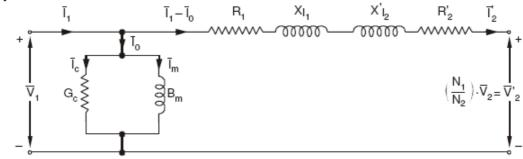
a. the exact model of a transformer.
