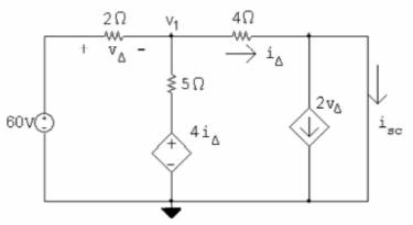
The node voltage equation:  $\frac{v_1 - 60}{2} + \frac{v_1 - 4i_{\Delta}}{5} + \frac{v_1}{4} = 0$ The constraint equation:
