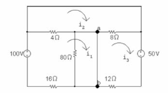
Note with the short circuit from a to b that  $i_{\Delta}$  is zero, hence  $124i_{\Delta}$  is also zero. The mesh currents are:
