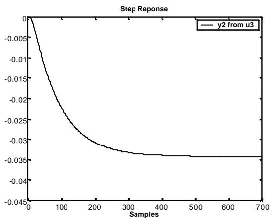
Figure 2.20: Unit step response of Output-2 from Input-3
