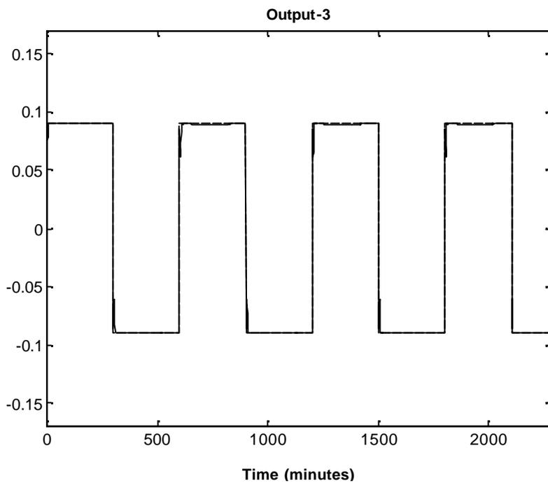
Figure 2.32: Tracking response of MPC to set point change (Output-3)
