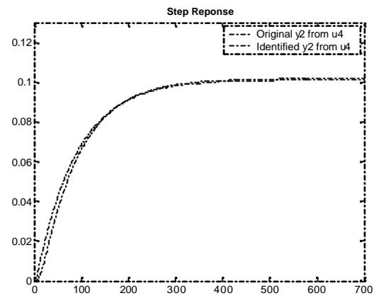
Figure 3.72 : Case 2- Step response of Output-2 from Input-4 (ARX)
