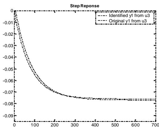
Figure 3.19 : Case 1- Step response of Output-1 from Input-3 (ARMAX)
