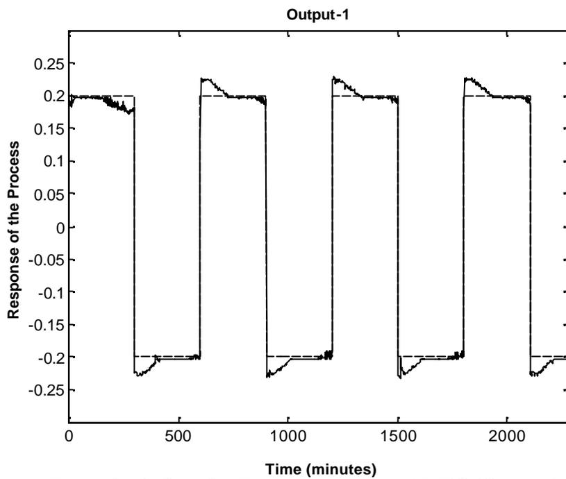
Figure 2.46: Case 2 - Tracking response of MPC (Output-1)
