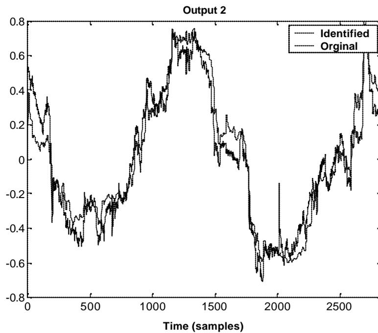
Figure 2.7: Open loop identified (dashed) and actual (solid) Output-2
