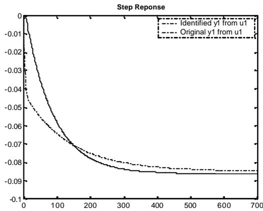
Figure 3.97 : Case 2- Step response of Output-1 from Input-1 (OE)
