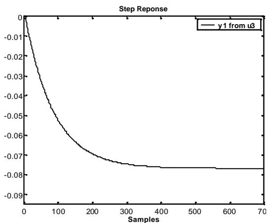
Figure 2.16: Unit step response of Output-1 from Input-3
