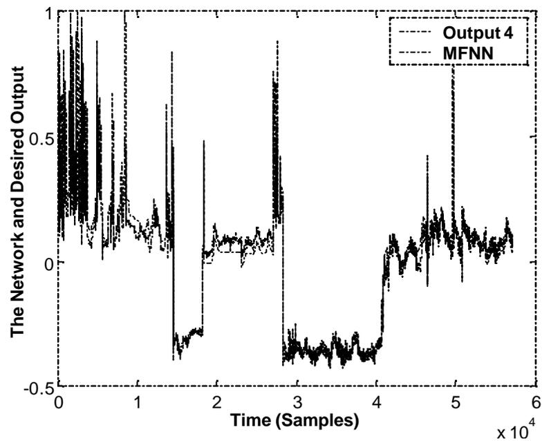
Figure 5.13 : MFNN and Desired Output 4 - Closed Loop Data
