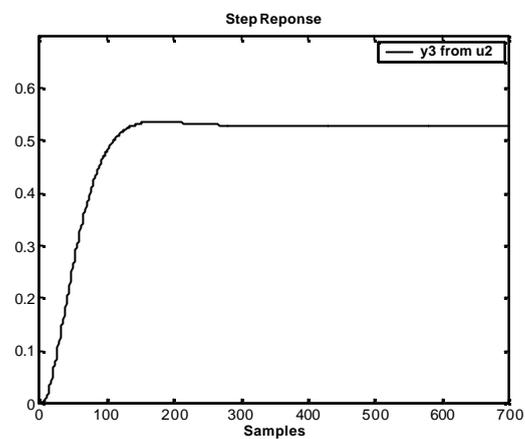
Figure 2.23: Unit step response of Output-3 from Input-2
