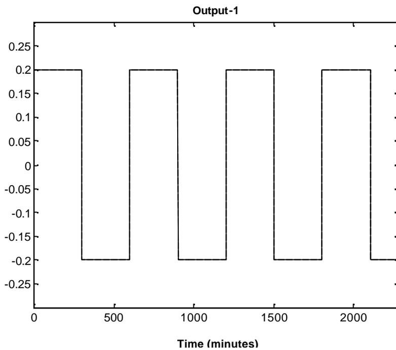
Figure 2.30: Tracking response of MPC to set point change (Output-1)
