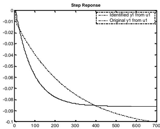
Figure 3.33 : Case 1- Step response of Output-1 from Input-1 (OE)
