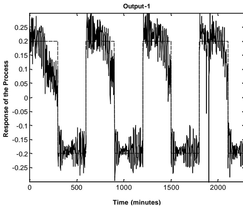
Figure 2.54: Case 3 - Tracking response of MPC (Output-1)
