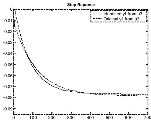
Figure 3.99 : Case 2- Step response of Output-1 from Input-3 (OE)
