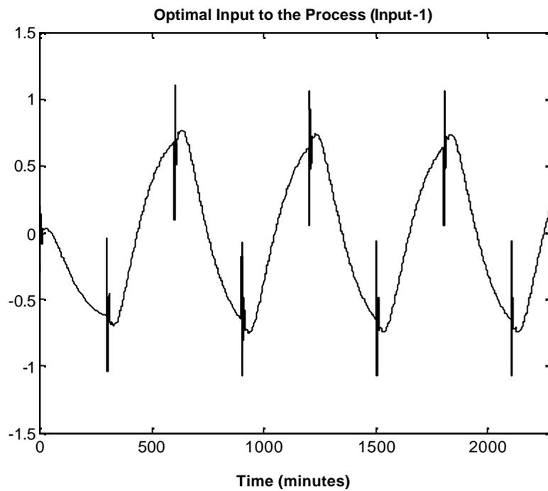
Figure 2.34: Optimal inputs generated by the MPC (Input-1)
