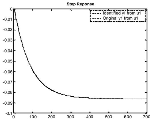
Figure 3.65 : Case 2- Step response of Output-1 from Input-1 (ARX)
