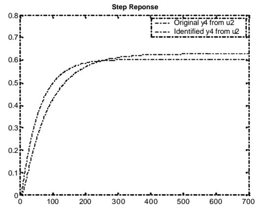
Figure 3.110 : Case 2- Step response of Output-4 from Input-2 (OE)
