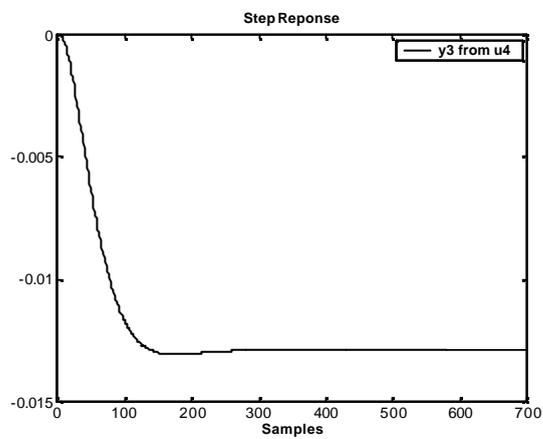
Figure 2.25: Unit step response of Output-3 from Input-4
