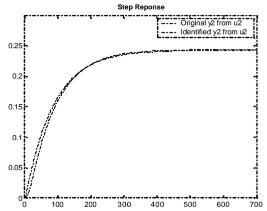
Figure 3.70 : Case 2- Step response of Output-2 from Input-2 (ARX)
