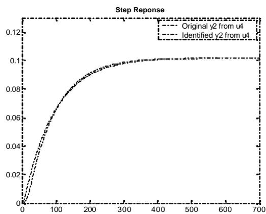
Figure 3.24 : Case 1- Step response of Output-2 from Input-4 (ARMAX)
