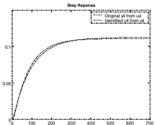
Figure 4.20 : Step Responses of the Actual Open Loop and Identified ARX models (Output-4 from Input-4)
