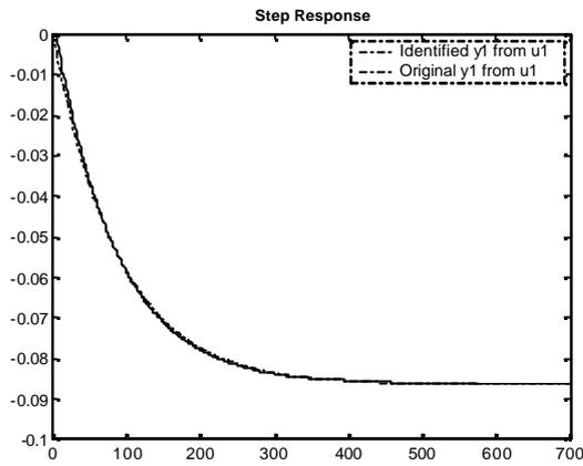
Figure 3.81 : Case 2- Step response of Output-1 from Input-1 (ARMAX)
