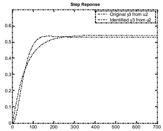
Figure 3.58 : Case 1- Step response of Output-3 from Input-2 (State space)
