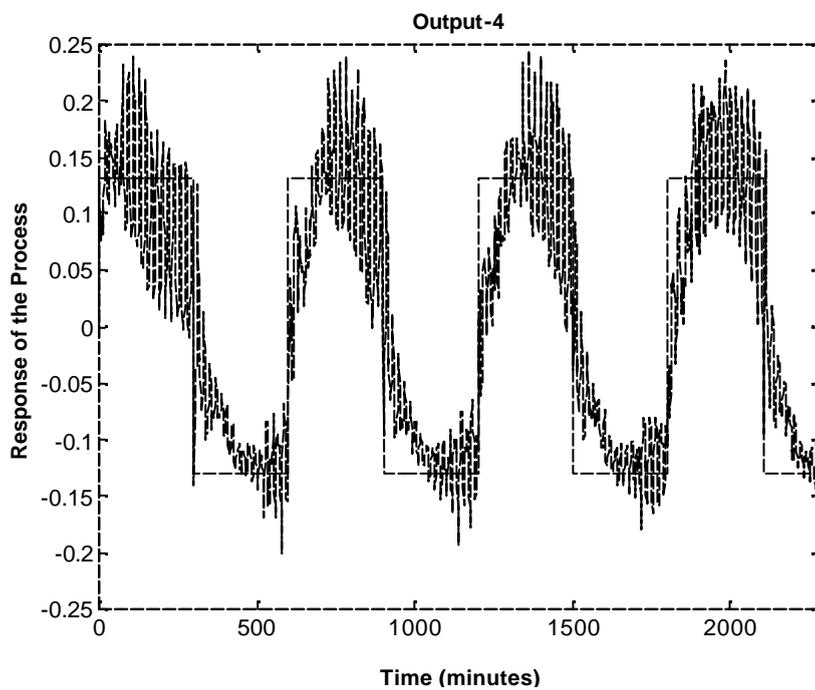
Figure 2.57: Case 3 - Tracking response of MPC (Output-4)
