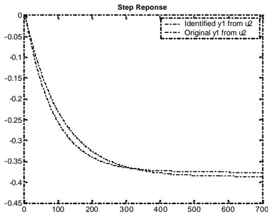
Figure 3.2 : Case 1- Step response of Output-1 from Input-2 (ARX)
