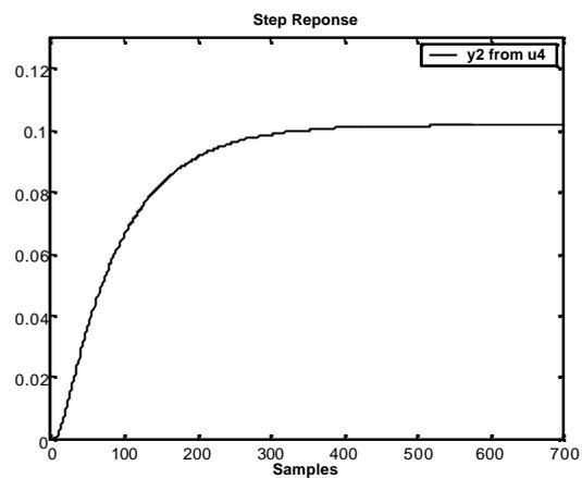
Figure 2.21: Unit step response of Output-2 from Input-4
