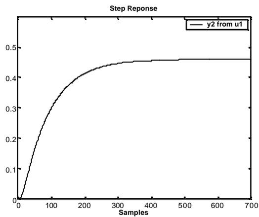
Figure 2.18: Unit step response of Output-2 from Input-1
