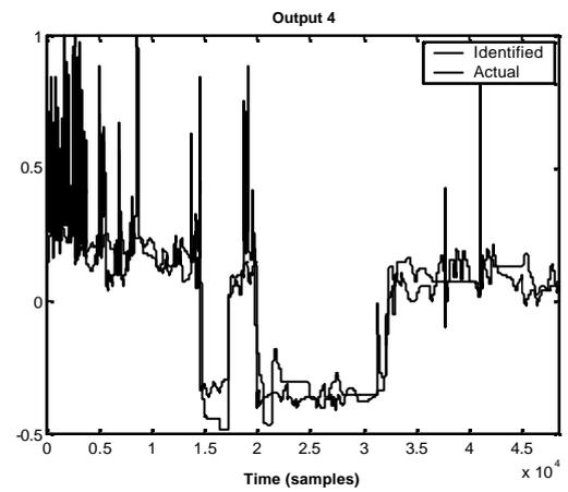
Figure 4.24: Responses of Output 4 Actual and Identified ARMAX Model
