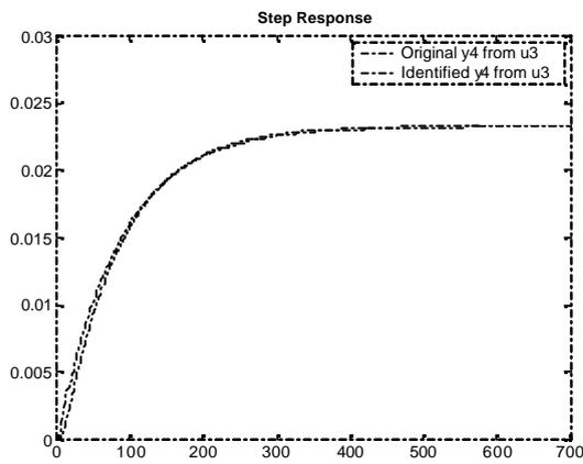
Figure 3.159 : Case 3- Step response of Output-4 from Input-3 (ARMAX)
