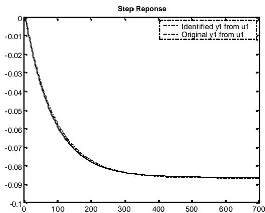
Figure 3.129 : Case 3- Step response of Output-1 from Input-1 (ARX)
