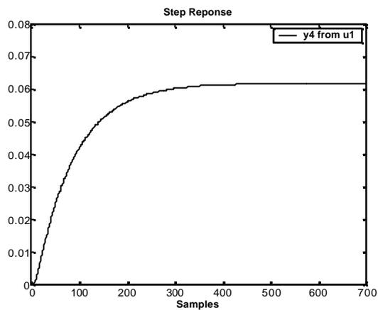
Figure 2.26: Unit step response of Output-4 from Input-1
