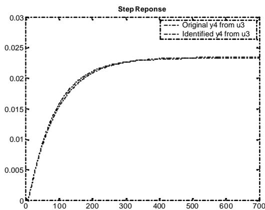
Figure 3.15 : Case 1- Step response of Output-4 from Input-3 (ARX)
