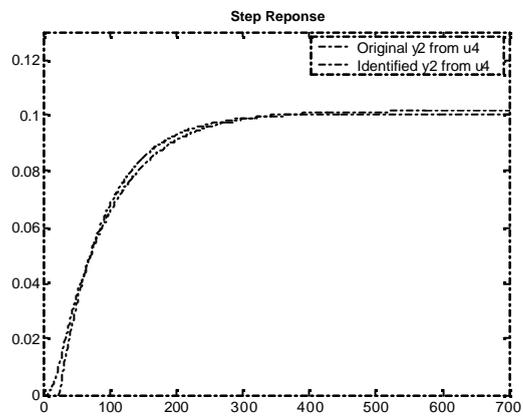
Figure 3.40 : Case 1- Step response of Output-2 from Input-4 (OE)
