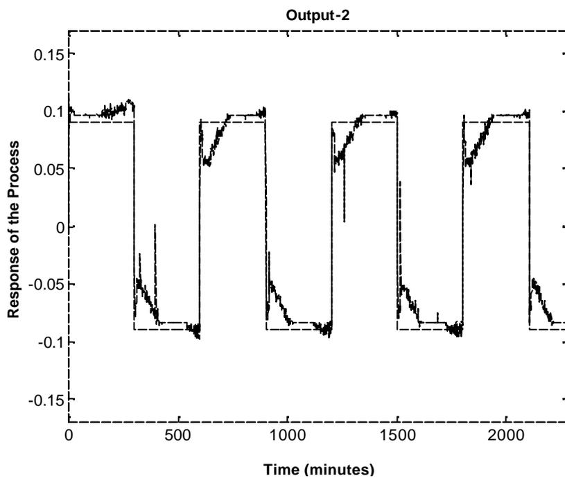
Figure 2.47: Case 2 - Tracking response of MPC (Output-2)
