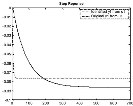
Figure 3.113 : Case 2- Step response of Output-1 from Input-1 (State space)
