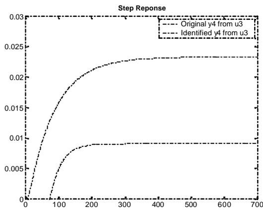
Figure 3.191 : Case 3- Step response of Output-4 from Input-3 (State space)
