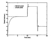
Fig. 4: Actual and desired speed of the DC motor for step changes
