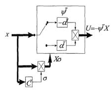
Fig. 1: Block diagram of variable structure controller
