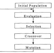
Fig. 2: Flow Chart for a Simple Genetic Algorithm
