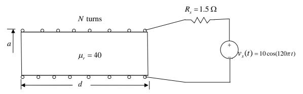
Design a suitable circuit (by calculating the number of turns N) that results in the maximum possible B field (maximum magnitude) inside the core of the solenoidal inductor.
