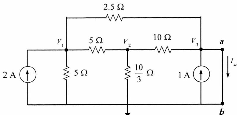
Here  $V_3 = 0$ , KCL on the two nodes  $V_1, V_2$
