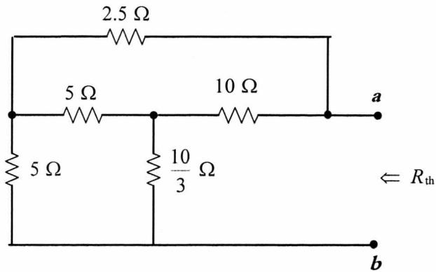
Since the resistors can not be combined as series and parallel, we then find  $R_{th}$
