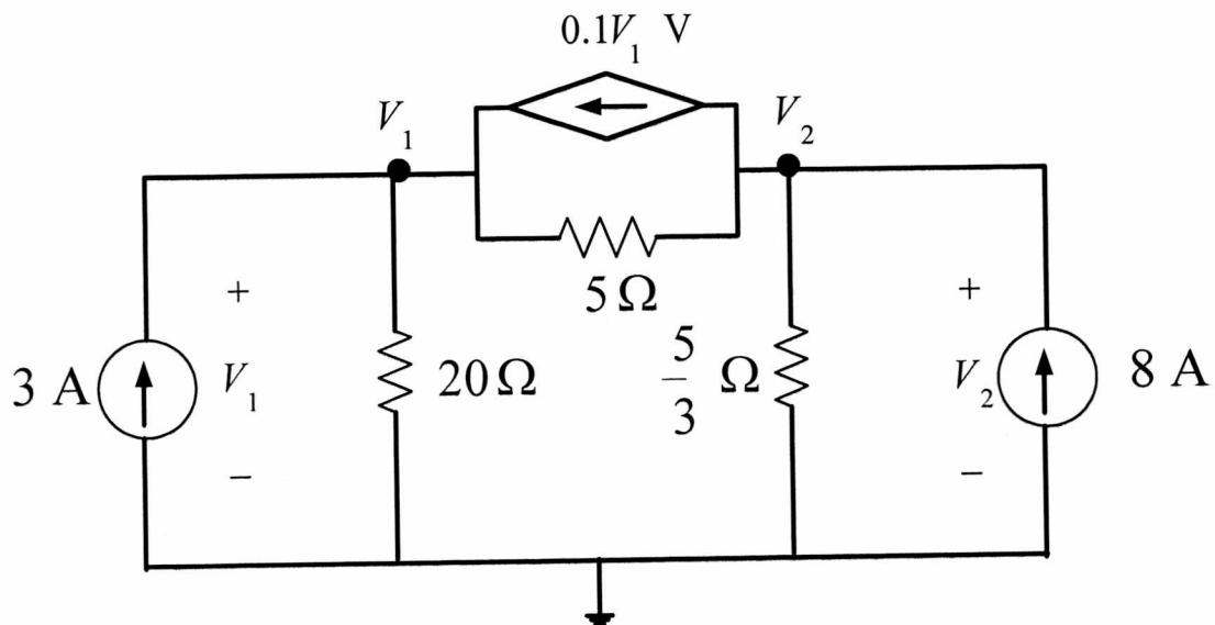
KCL on the two nodes  $V_1$ ,  $V_2$ , we have
