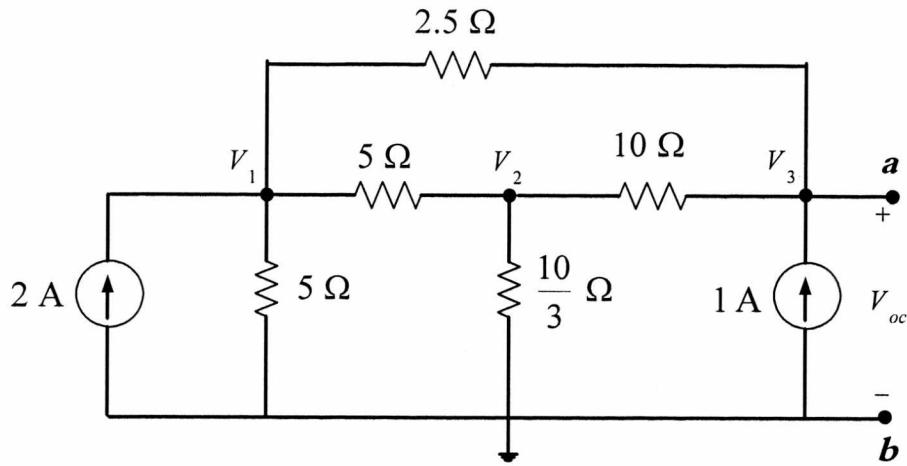
KCL on the three nodes  $V_1, V_2, V_3$
