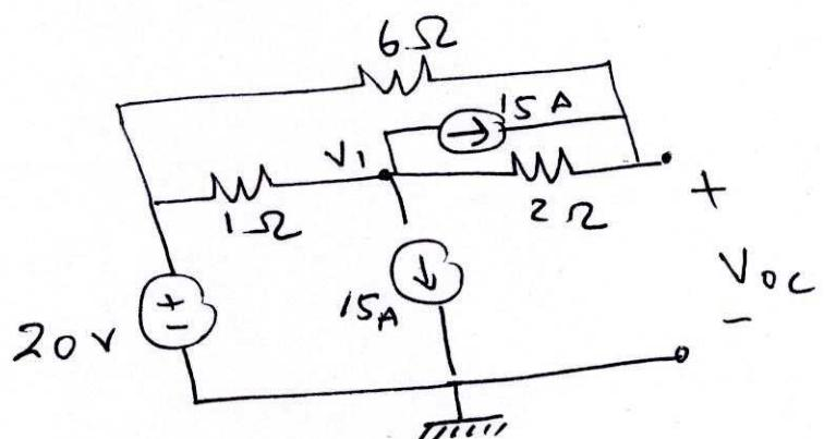
using Nodal analysis to find  $V_{oc}$
