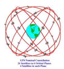
GPS user community in terms of obtaining accurate data up to about 100 meters for navigation, meter-level for mapping, and down to millimeter level for geodetic positioning. The GPS NAVSTAR (Navigation Satellite Timing and Ranging Global Positioning System) is a satellite-based navigation, timing and positioning system (1).
