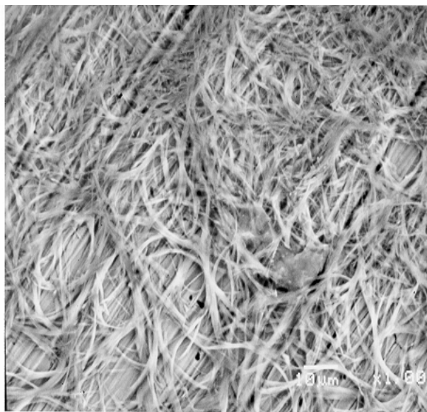
Figure 8. SEM micrograph taken on the white layer of the unexposed steel specimen treated with 100 mM sodium benzoate.
