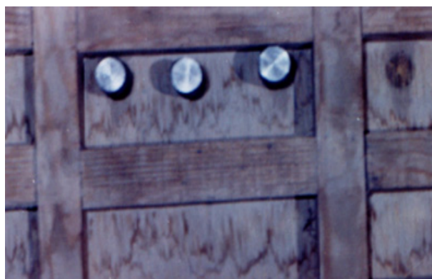
Figure 4. Photograph of steel specimens exposed to atmosphere for a month after treatment with 100 mM sodium benzoate.
