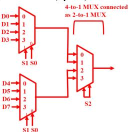
Grading: Three 4-1 MUXs in the shape of a tree=1 point. Correct selection lines and data lines=1 point. Correct 4-1 as 2-1=1 point. Using incorrect MUX size=-0.5. Missing data line labels -0.5 for every MUX. Missing selection line labels -0.5 for every MUX, except when it does not matter, like the MUX in the right.
