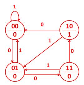
**Part II:** The following state diagram is for a sequential circuit with input x, output z, two state variables A and B, **positive** edge-triggered flip-flops, and **asynchronous active HI** reset.
