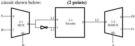
Inputs are A and B, and outputs are F0 and F1. Derive the truth table for this circuit. Hint: It helps if you evaluate the internal signals, L1 and L2, before evaluating the outputs.
