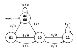
a) Complete the timing diagram below for the above state diagram, showing the waveforms of the state variables A and B, and the output z. Initially, the flip-flops are reset to A = B = 0. (4 points)
