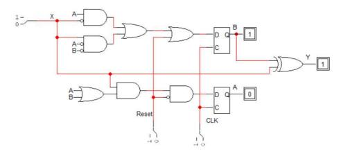
**b**) (6 points) It is required to write a **behavioral** Verilog module to model the given sequential circuit. Complete the given Verilog code to achieve that.
