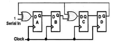
(2 points) Consider the given synchronous counter circuit. The LOAD input is synchronous and the Clear (reset to 0) input is asynchronous. Initially one short 0 pulse is applied at the clear input. The circuit implements a modulo-\_\_\_\_\_ counter. With a clock input signal having a frequency of 720 cycles/sec, the frequency at the output signal is \_\_\_\_\_ cycles/sec.
